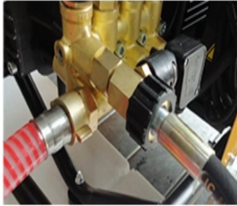
2. Machine connected to the inlet and outlet pipes
